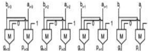
Fig 7: Generation of propagate and generate bits
